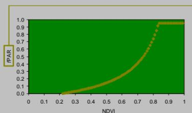
Figure 2. Relationship used to derive  $fPAR$  from MODIS NDVI.
